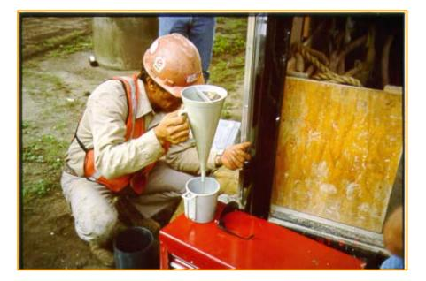
Figure A-13: Marsh Funnel Viscosity Test
