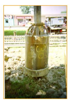
Figure A-1: Drilled Shaft Cleanout Bucket
