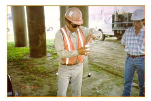
Figure A-14: Testing the slurry for sand content
