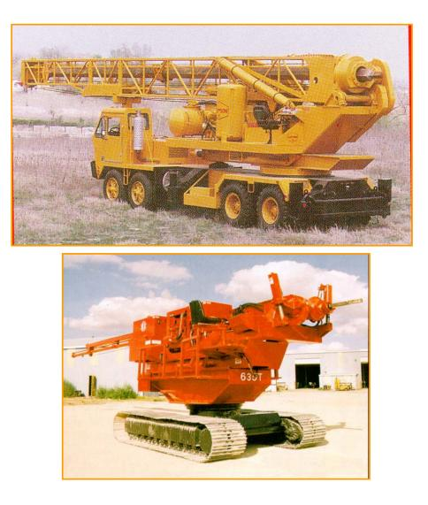
Figure A-22: Two types of Drilled Shaft Foundation Construction Equipment.
