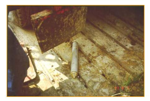
Figure A-12: Cone Slurry Density sampler.
