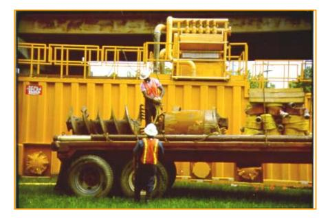
Figure A-6: Slurry Tank(yellow tank) & Desander .The desander is the device that looks like an engine on the top of the tank. Notice the auger and cleanout bucket being unloaded off the truck.
