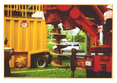
Figure A-2: Drilled Shaft Soil Auger or Flight Auger
